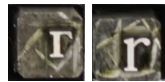
Figure 18. “0.2 inch composition punches for Imprint Bold (typeface series number: 310), font size 8”, Monotype Corporation Collection, Science Museum object co8725570 , showing two variants of capital r with long leg.
