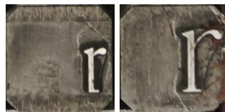
Figure 20. “0.4 inch composition punches for Imprint (typeface series number: 101), font size 18”, Monotype Corporation Collection, Science Museum object co8723829 , showing small and capital r with long leg.
