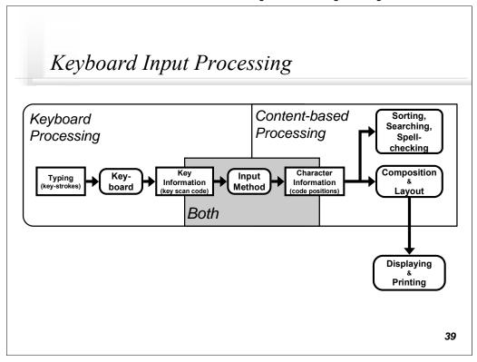
Let's examine a model for keyboard input. This model, in some ways, is an overlay of the Key and Character domains in the earlier figure. Note the input method area of processing is in both the key and the character domains.
