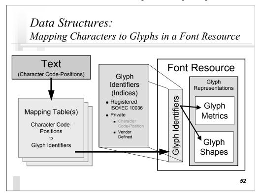
If glyph identifiers, either registered or vendor defined, are used, glyph selection requires tables to map from the character code position into the glyph identifier used to index into the font resource to obtain the glyph metrics and glyph shapes. The mapping tables may implement one-to-one mappings or more sophisticated *M*-to-*N* mappings.
