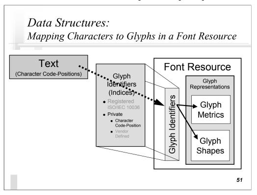
If the private, character code position is used for the glyph identifiers, glyph selection is one-to-one and consists of using the code position for a character to index into the font resource to obtain the glyph metrics and glyph shapes.
