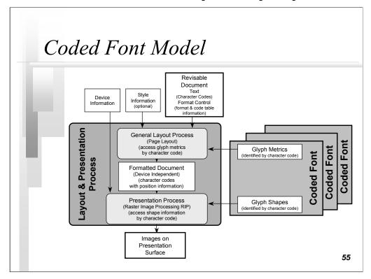
A coded font (or a character-coded font) is a data structure in which character codes are used to index the glyph metric and glyph shape information contained in the font. The data structure depends on a one-to-one mapping of character codes to the glyphs in a font. Note that each code supported requires a separate coded font even if the glyphs are the same.
