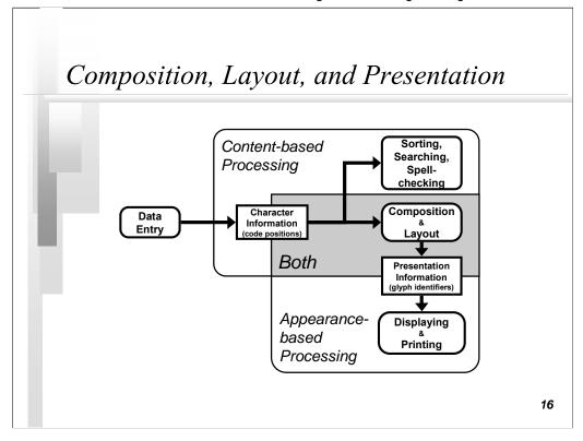
Let's examine another model for the composition, layout, and presentation functions that you will find in a wordprocessor. This model, in some ways, is an overlay of the domains of previous figure. However, it is interesting because of an area of processing that is in both the character and the glyph domains.
