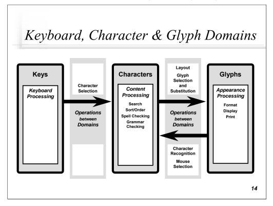
This figure shows three distinct domains, one for keys on keyboards on the left, one for characters in the middle, and another for glyphs on the right. It also uses arrows to show operations for going from one domain to the other. Note that the character domain provides the common mechanism for taking the keys on the keyboard and displaying the resulting glyphs.
