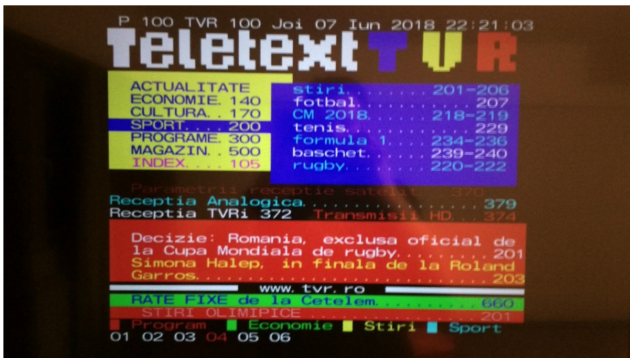
Figure 12. A present-day example of digital teletext in Romania, using block semigraphics from the teletext character set. (Ricardo Bánffy)
