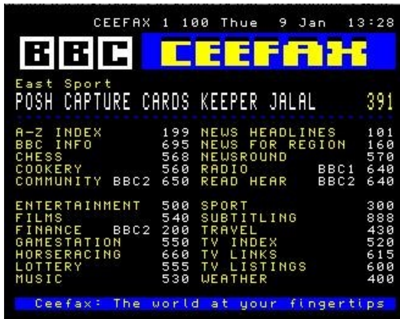
Figure 10. Screen shot from CeeFax, the world’s first teletext information service. Note the use of foreground and background colors, double-height text, and semigraphics.
